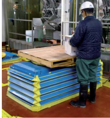
Use electric or pneumatic scissors lift (accordion skirting).
