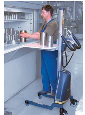
Adjust the load lifter to shelf level and remove containers by sliding them out.
