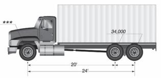
This vehicle has a bridge of 24' between axles 1 and 3. Using the B/F chart, this vehicle would be allowed a gross weight of 54,000 lbs. If this vehicle exceeds the B/F gross weight of 54,000 lbs., the vehicle does not qualify for the bridge formula so only designated weights would apply.
