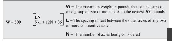
A Bridge Gross Weight Formula chart is provided on page 41 of the *Truck Driver's Guidebook*. The chart is an easy means of determining permissible gross loads for vehicles in regular operation.
