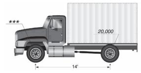
This vehicle has a bridge of 14'. Using the B/F chart, check the distance of 14' for two axles, finding a gross weight of 40,000 lbs. If this vehicle exceeds the formula weight of 40,000 lbs., the vehicle does not qualify for the bridge formula so only designated weights would apply.
