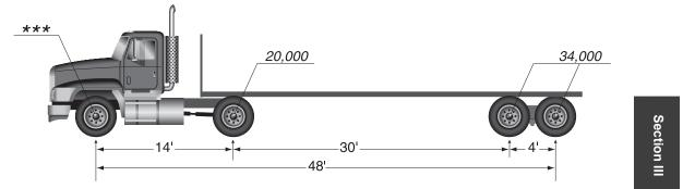
This combination has a bridge of 48' between axles 1 and 4. Using the B/F chart, this combination would be allowed a gross weight of 74,000 lbs. If the combination exceeds the B/F gross of 74,000 lbs., it would not qualify for bridge formula weights so only designated weights would apply (up to 18,000 lbs. on a single axle/16,000 lbs. for each axle on the tandem, with proper tire sizes).
