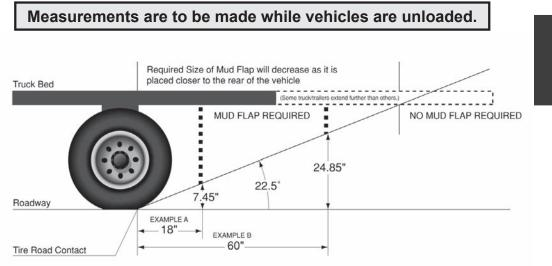
The above diagram can be used as a guide in determining whether your vehicle is required to have mud guards or flaps. Compliance may be determined by whether the rear wheels of a commercial vehicle throw road surface substances back and up at an angle greater than 22.5 degrees.
