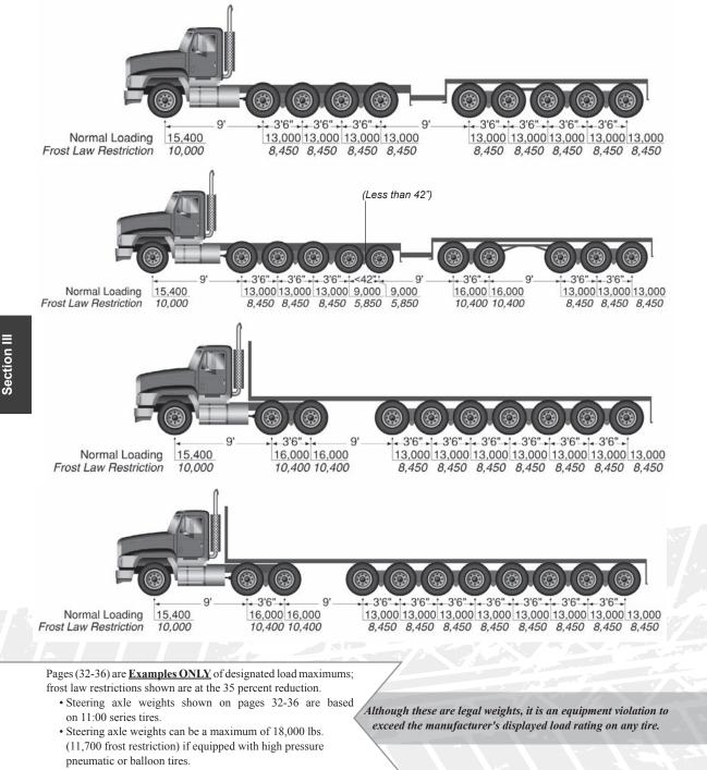
The Bridge Gross Weight Formula was developed to prevent stress to highway bridges caused by heavy trucks. The formula provides a standard to control the spacing of truck axles and weight on those axles. Vehicles with a gross weight of 80,000 pounds or less may be eligible for increased weights using the Bridge Gross Weight Formula. Vehicles exceeding a gross weight of 80,000 pounds or the gross weight calculated using the Bridge Weight Formula **are not eligible** for bridge weights.
